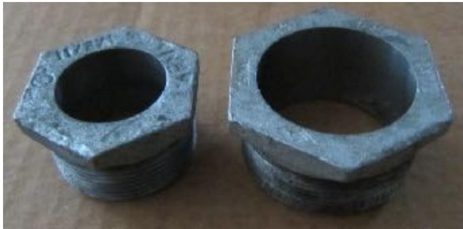
*NOTE: Grind out the bushing's threads until the Inner Pole slips freely through.*
