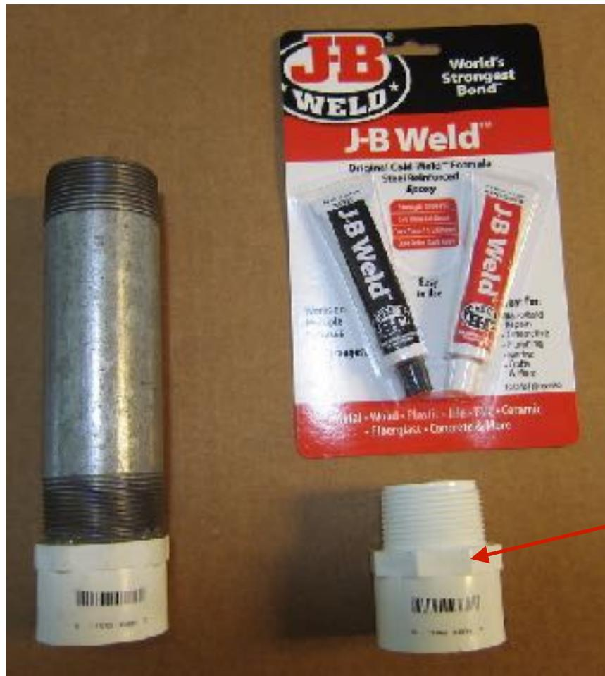
Some of the slack of the inner telescoping pole can be removed by adding a Centralizer to the bottom of the pole. A 1 1/4" PVC Male Adapter can be driven into the bottom of the pole and secured with JB Weld or equivalent. File down enough of the PVC points to allow the pole to slide smoothly inside the 2" outer pole.
